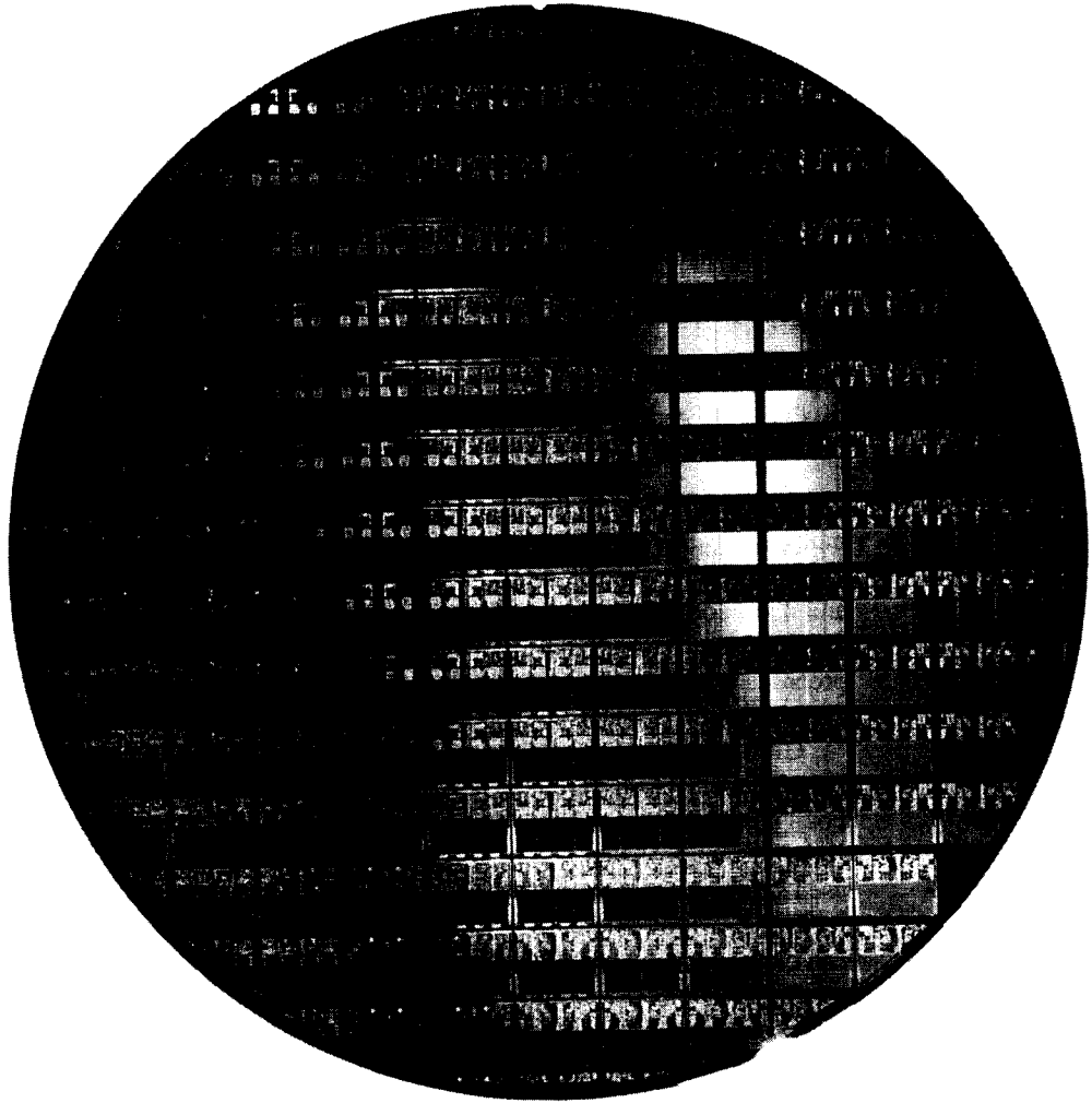
Figure 1.12 This 300mm wafer contains 117 AMD Opteron chips implemented in a 90 nm process. (Courtesy AMD.)
